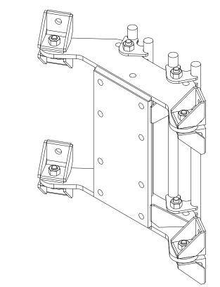
DETAIL D FOR TRI-LOCKNUT INSTALLATION, ENSURE GROOVED SIDE IS ORIENTED AWAY FROM THE BOLT HEAD
